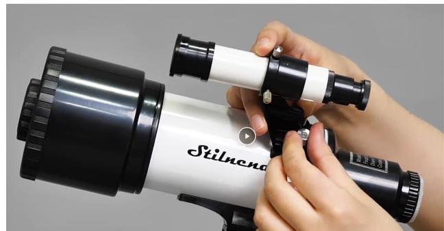
4. Install the eyepiece of choice into the Zenith Mirror
